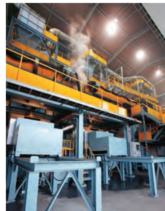
A machine for reducing the volume of shredder dust and solidifying it
