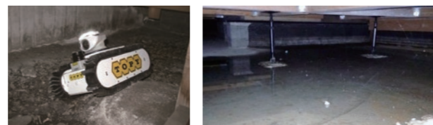
Inspection of flooded houses under floor in heavy rain disaster
