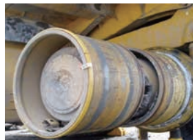
Tire change in progress (Tires can be changed without removing the wheel from the mining vehicle)
