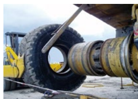
Tire change in progress (Tires can be changed without removing the wheel from the mining vehicle)
