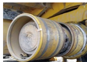
Tire change in progress (Tires can be changed without removing the wheel from the mining vehicle)
