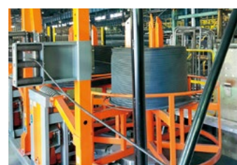
Densely rolled compact coil is drawn and put into the NC processor
