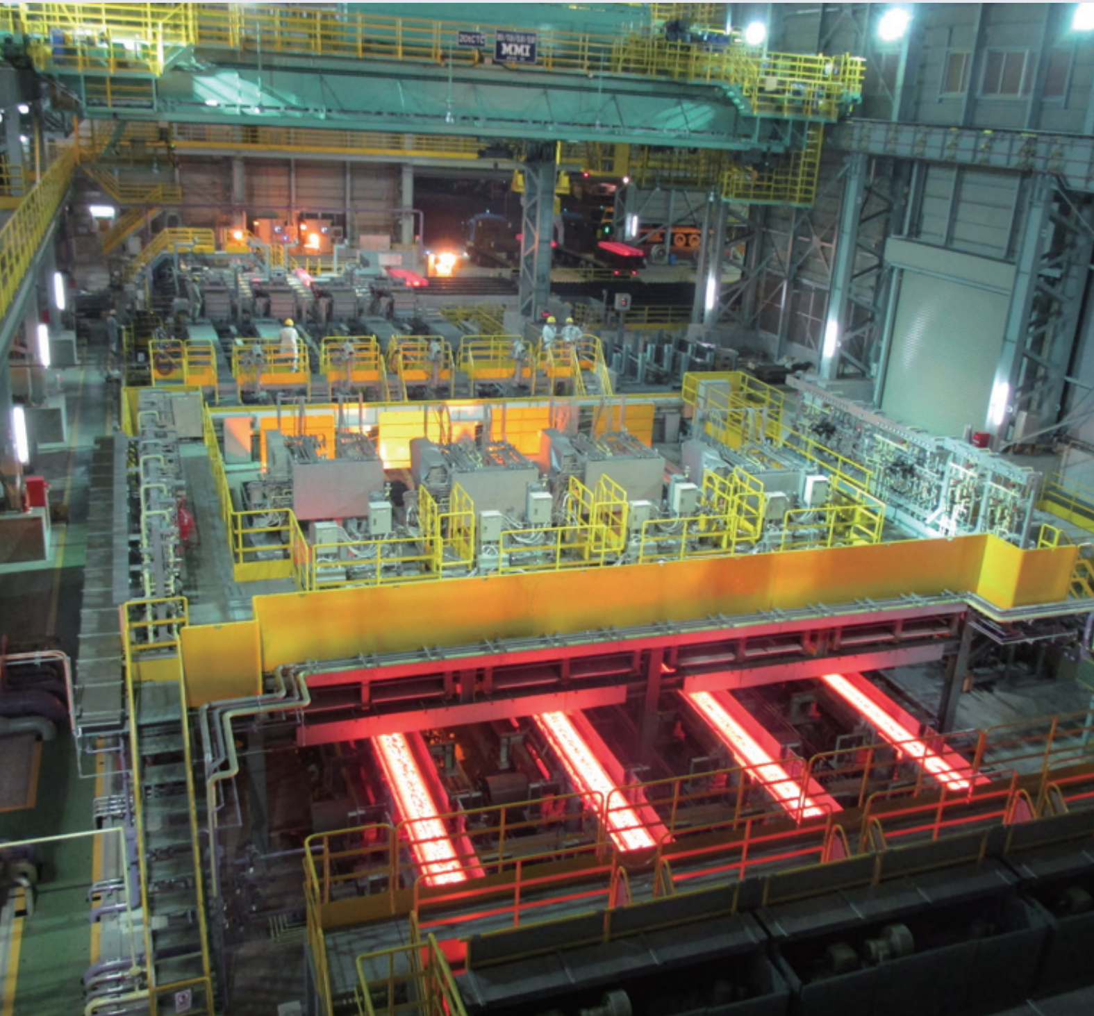
A Continuous Casting Machine at New Steel Making Facilities, Toyohashi Factory
