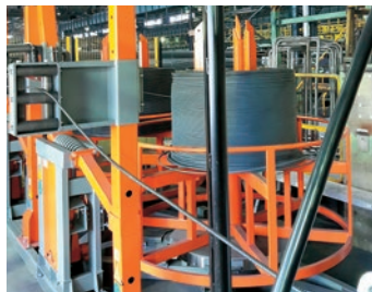
Densely rolled compact coil is drawn and put into the NC processor.
